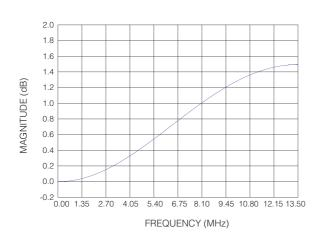
Fig. 7 SIN X/X Compensation Filter Frequency Response (Sampling at *f* s=27MHz)
