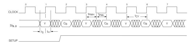
Fig. 10 Operation of SETUP Control Signal
