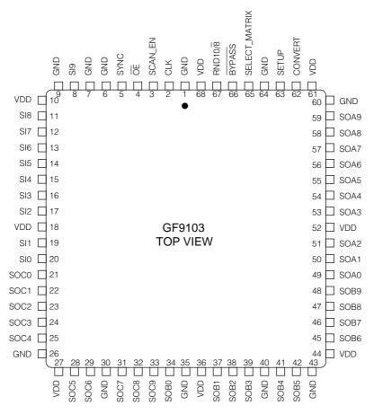
Fig. 1 GF9103 Pin Connections
