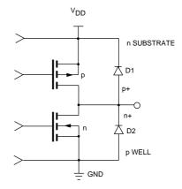
Fig. 2b Equivalent Output Circuit
