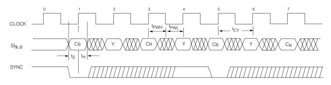
Fig. 9 Operation of SYNC Control Signal
