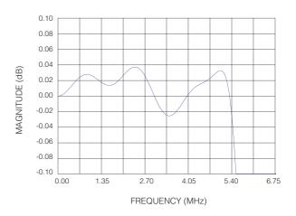
Fig. 4 Frequency Response of Luminance Interpolation Filter (Sampling at *fs*=27MHz)
