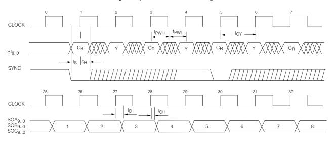
Fig. 11 Input/Output Timing, BYPASS = 1
